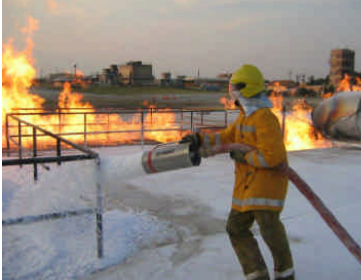
Angus Tridol ATF medium expansion foam controls LNG spill fire
