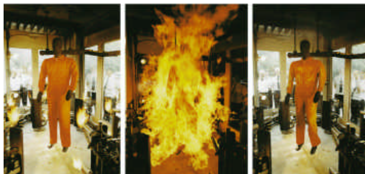
DuPont's Thermo-Man® testing system evaluates the protective performance of PPE.
