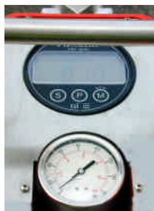
Residual pressure on gauge and digital readout of flow.
