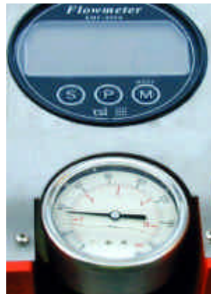
Static pressure reading on pressure gauge
