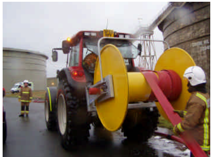
SVT Demo236 Valtra Tractor fitted with hose recovery reel. BP Sullom Voe Oil Terminal
