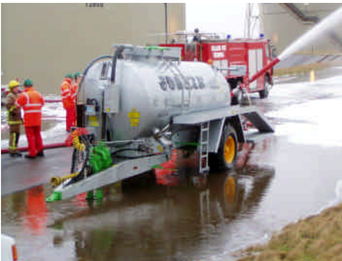
SVT Demo203 8,400 litre Foam Tanker with POK monitor in operation. BP Sullom Voe Oil Terminal
